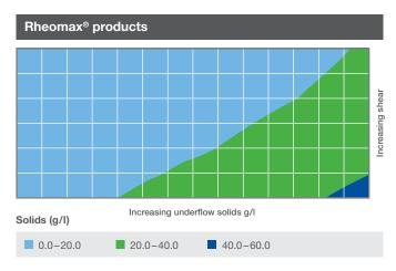
The Rheomax® DR range of products produce an underflow with a lower yield stress, which is more tolerant to fluctuations in solids content and applied shear, resulting in a more consistent thickener performance over a wide range of operating parameters.
