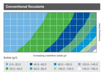
Conventional flocculants are sensitive to fluctuations in solids content and applied shear, which can limit their associated process performance. The graph shows the effect on yield stress as plant conditions vary.
